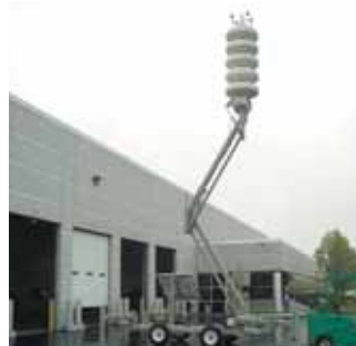
This custom designed siren lift and trailer raises a 10 ft. tall, 4 ft dia., 1000# siren, 27 ft. into the air and is capable of withstanding winds of 100 mph in the raised position.
