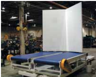
This lift has 60,000 lbs. of capacity and has a 9 ft. by 35 ft. platform. Similar units have been built with platforms as long as 60 feet.
