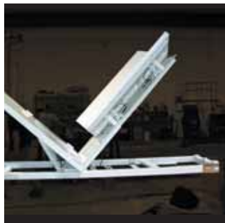
These custom designed tilters handle 5000# rolls of tissue, 8 ft. in dia. by 8 ft. long. The unit on the left has a fixed "V" cradle and powered conveyor flat deck. The companion unit on the right has a hydraulically adjustable "V" cradle for handling rolls of the same size.
