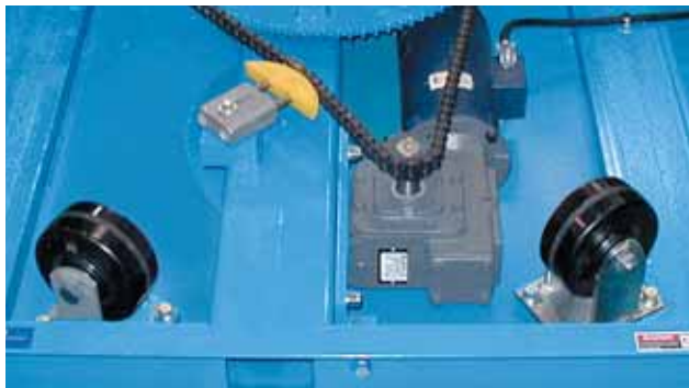
▶ Lifetime lubricated roller bearing wheel style of unit
