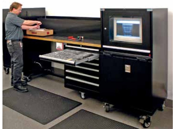
A mobile computer cabinet is paired with a mobile industrial workbench in Toyota Racing Development's machine shop.
