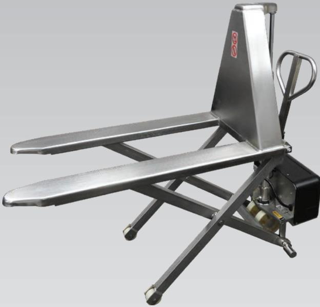
The Maxx-Jack Electric High Lift Stainless-Steel (MJHLE-SS) is perfect for lifting skids, plastic pallets, wire baskets, and open bottom containers in the food, beverage, and pharmaceutical industries. The 12V electrical system includes a battery and remote charger. The standard automatic floor lock prevents the unit from moving while in the raised position.
