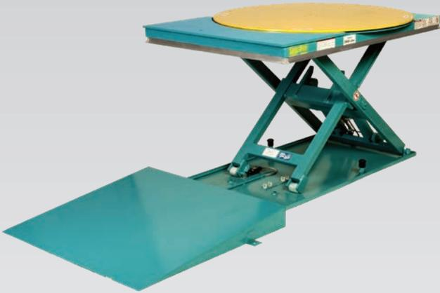
The Guardian Lift N' Spin Scissor Table (LPBL-LS) is an ergonomically designed workstation designed for the operator's health, safety, and comfort. Like the Guardian Low Profile table, The Lift N' Spin has an added workstation benefit of a 45" diameter rotating top. With a lowered height of 4.25" and our exclusive auto transition plate, the Lift N' Spin is quickly loaded. This low-profile table has a load capacity of 2,000lb and a 30.75" vertical travel, delivering an excellent lift table value.
