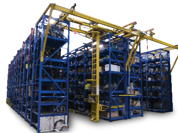
HEAVY PALLET STORAGE & RETRIEVAL SYSTEMS (STAK SYSTEM)
