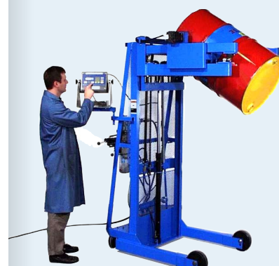
Scale-equipped to dispense measured amount from a drum
