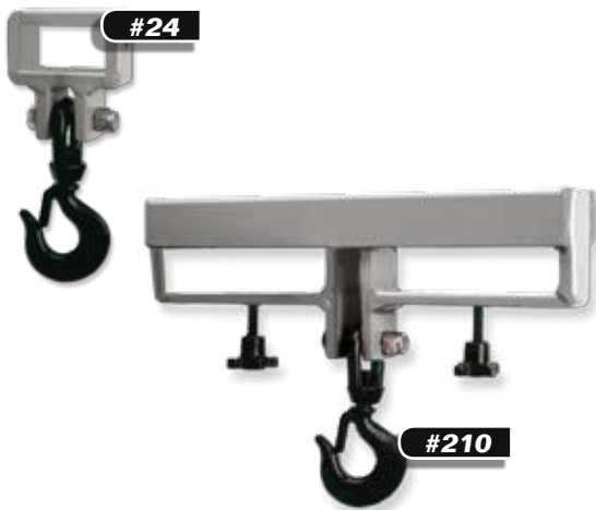
#24, #25, #26 & #210 - Easy handling by one person. In seconds the hooks can be slid on and tightened into place. Removes just as easily, no wrenches required. No. 210 Double Fork Hook has maximum openings, which permit an outside fork spread of 20-3/4". Capacity: Single fork - 3,000 lbs, Double fork - 4,200 lbs.
