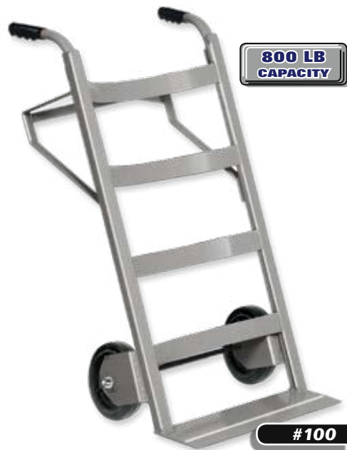
#100 Barrel & Drum Truck - Tubular construction with ball bearing mold-on rubber wheels, absorb shock, provide easy handling and quiet operation. Polymer grip handles. Balanced load exerted on the axle, bearings and wheels, and off the operators arms and shoulders. Dimensions: 42" H, 20" W, Toe Plate 5" x 19" Wheels: 8" x 2" mold-on rubber wheels Capacity: 800 lbs. Weight: 58 lbs.
