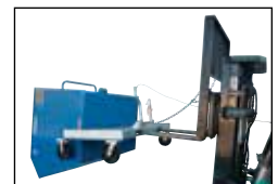
Hopper must be attached to a fork truck when dumping.
